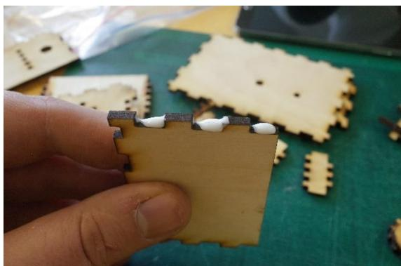
Start by gluing the sides to the top panel.
