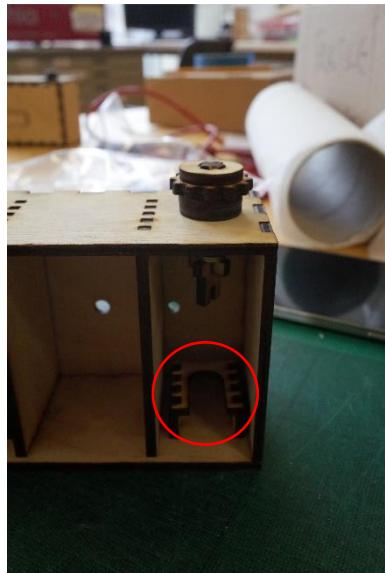
Glue the side and front panels to the bottom panel. Make sure the front is on the correct way with the text at the bottom.
