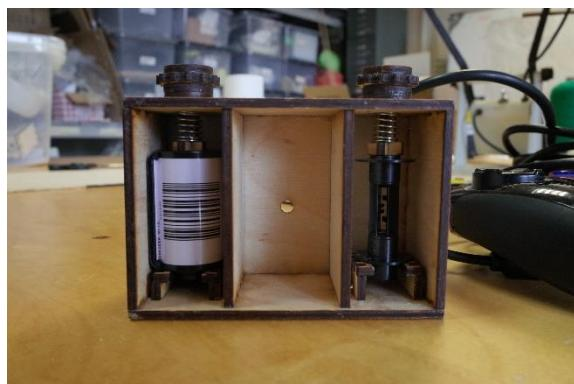
Finally we'll tape in the pinhole, epoxy the tripod bolt to the bottom of the outer case and attach the shutter with a nut and bolt and the camera is ready to use.
